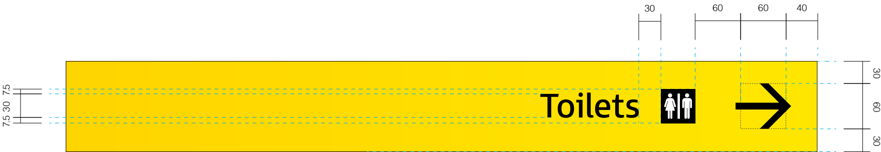
Typical Single Panel Arrow, Destination & Pictogram Scale 1:5
