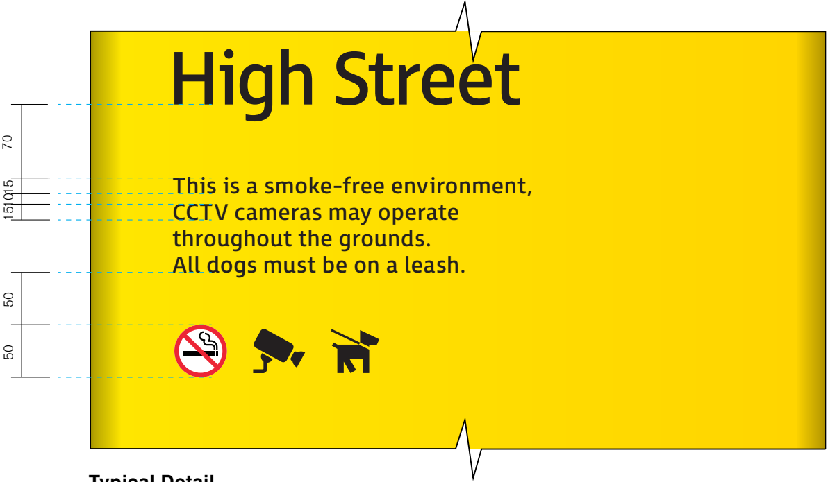
Typical Detail Regulatory messaging Scale 1:5
