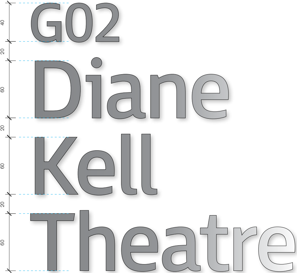
02 Detail Scale 1:2 Spec Lettering as 3mm thk lasercut aluminium with No. 4 finished stainless steel finish, adhesive fixed to door surface. Contractor to ensure surface is appropriate for adhesive fixings.
