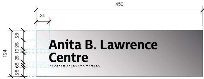
05 Detail Braille Panel Scale 1:5 Spec Panel as 10mm thk aluminium with No. 4 linished stainless steel finish, conceal fixed to wall with 5mm shadow gap as shown. Contractor to advise fixing method. Messaging as raised tactile matte black lettering.
