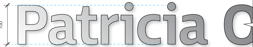
05 Detail Heading Scale 1:5 Spec Lettering as 5mm thk lasercut aluminium with No. 4 finished stainless steel finish, adhesive fixed to wall surface. Contractor to ensure surface is appropriate for adhesive fixings.
